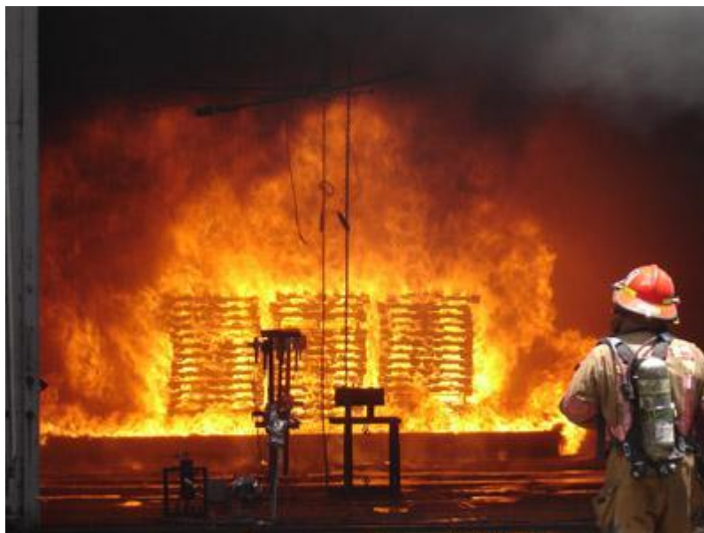
Researchers conduct well deck fire suppression tests. (Photo Credit: Naval Research Laboratory)
